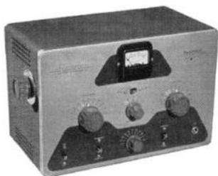
Heathkit DX-20. This was a crystal controlled, 80 through 10 meter rig that ran 50 watts input on CW only.
